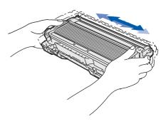
4 Put the drum unit assembly into the machine until it clicks into place.
